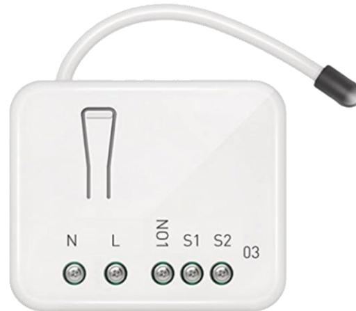
The Quadrobit relays allow you to control the wall switch, the lighting zone or the built-in socket using the QUADROBASE HUB. This small module is installed in the electrical box behind your switch/socket, namely the breaking of the wire circuit of the power supply socket. When the module is installed, the wall switch will work as before from the hand (mechanically) and from the Quadrobit application in your phone.
