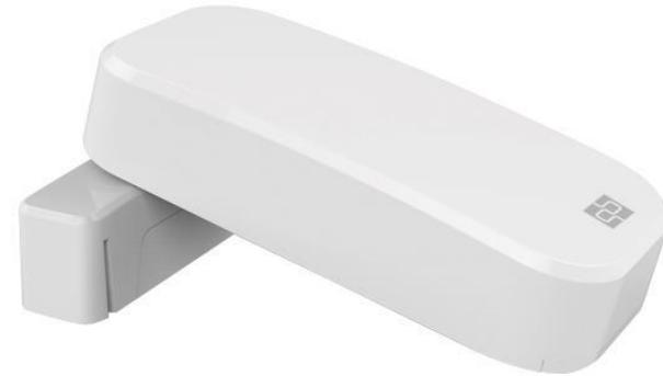
The battery powered wireless door/window sensor is designed to detect the opening of doors, windows, hatches, gates. The sensor consists of a magnet and a sensor (reed switch), which determines the change in the magnetic field. When the magnet moves away from the sensor, the detector detects the change and sends a signal to the device to which it is connected.
